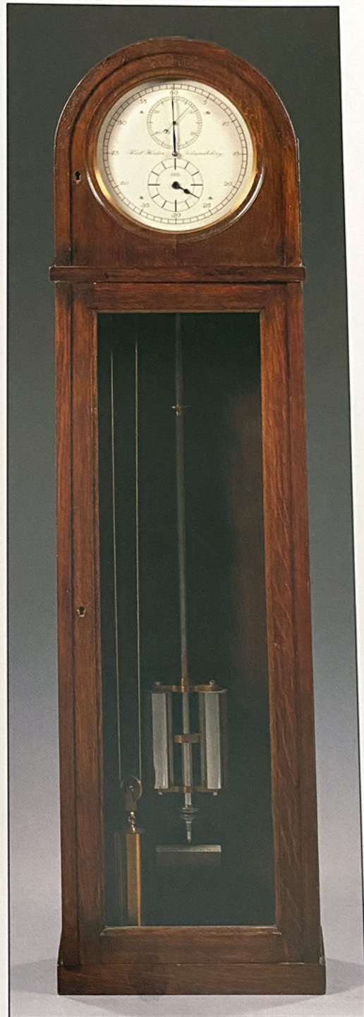
Fig. 34-22. Strasser & Rhode, Glashütte, dated on the dial 1935 and signed there by Karl Hanker. It has a dead beat escapement, adjustable jeweled pallets, jeweled pivot holes for the escape wheel and pallet arbors, wheelwork with five crossings, maintaining power and a weight offset to one side. It has Strasser's two cylinder nickel-steel pendulum and his own form of spring impulse escapement. Case Style 15.
