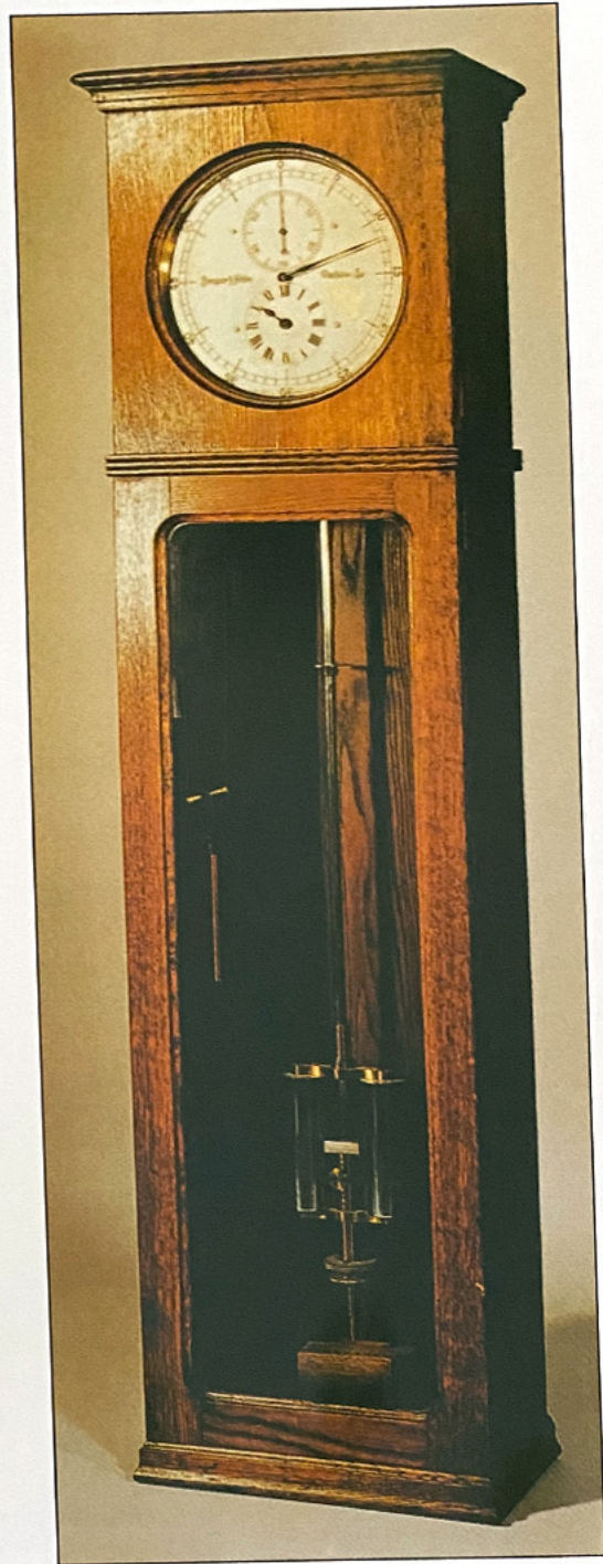
Fig. 34-18. Strasser & Rohde. A Style 5 oak cased wall regulator with Type 13 pendulum with adjustable compensation unit between the cylinders and Graham dead beat escapement with jeweled pallets.
