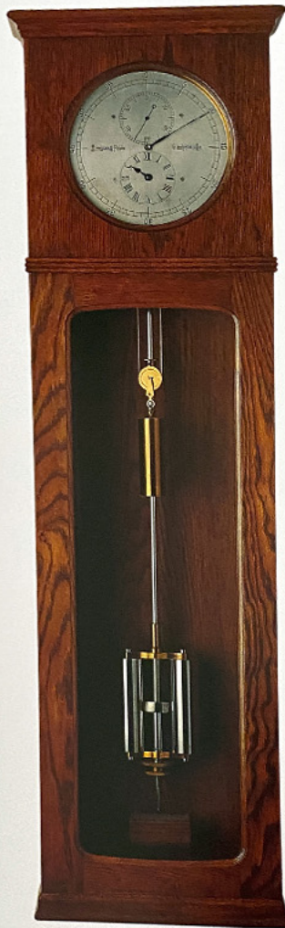
Fig. 34-19. Strasser & Rohde, Glashütte i/Sa. It has an oak case, dead beat escapement with sapphire pallets and chatons for the sapphire pivot holes for the escape wheel and pallet arbors. The compensating unit between the twin bobs may be adjusted. The case is a slightly modified Style 5.
