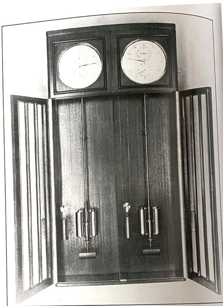
Fig. 34-25. Strasser & Rohde Nos. 917 and 918. These two regulators, one showing sidereal and the other mean-time, were made for the observatory in Stalingrad and housed in this specially designed double case. One wonders whether the proximity of two pendulums, within one case, beating at different rates, would have affected their performance.
