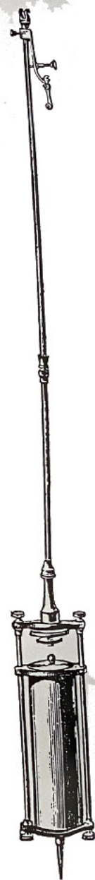
Fig. 34-8F. Mercury compensated pendulum based on the Glashütte design. It has a cast iron jar with screw-on lid. The length of the column of mercury was calculated at 144mm.
