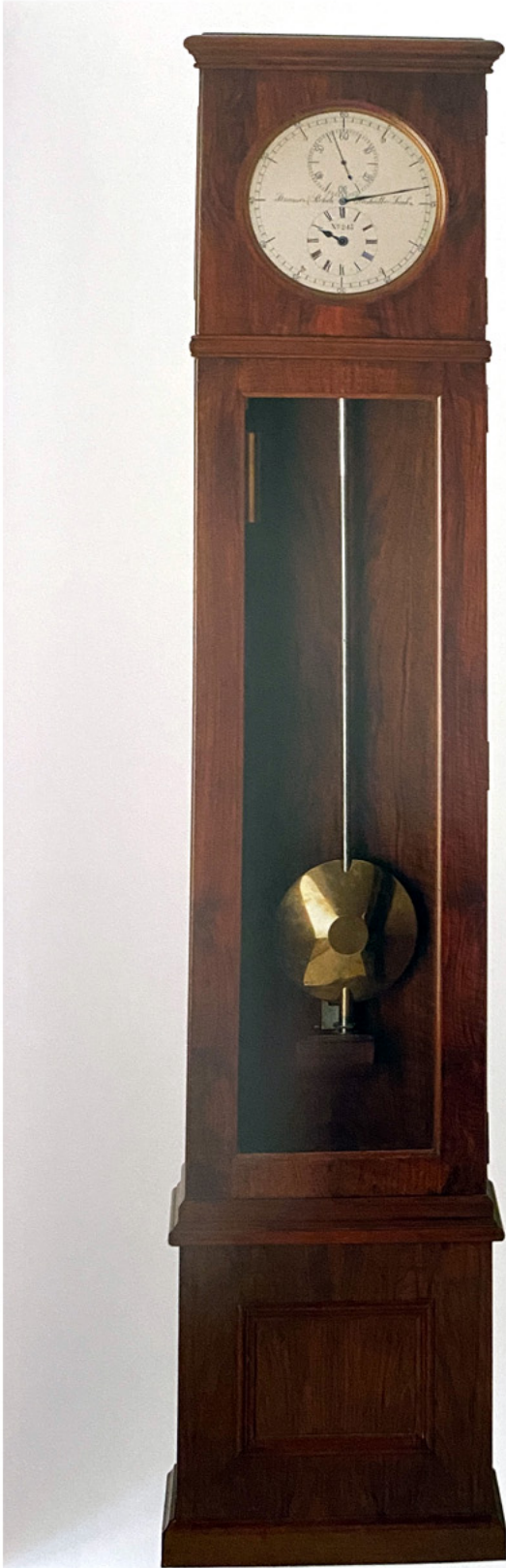
Fig. 34-10. Strasser & Rohde, No. 245. This walnut regulator with Strasser's escapement has an offset weight, ruby pallets, and the escape wheel and pallet arbors running in jeweled pivot holes. Riefler's Invar compensated pendulum is employed.
