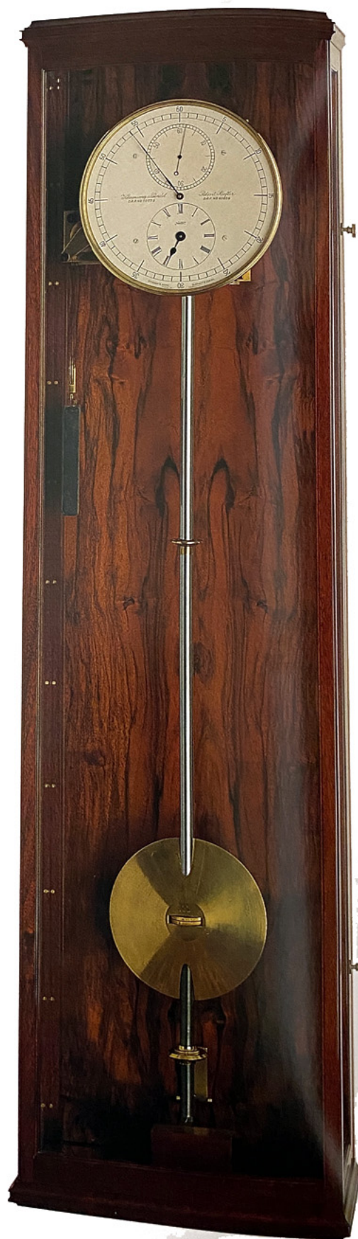
Fig. 34-9. Strasser & Rohde, Glashütte i Sachsen. Pendulum Patent Riefler, D.R.P. No. 50739, D.R.P. 60059, c. 1897. An early weight-driven rosewood wall regulator with Riefler's mercury compensated pendulum and Strasser's form of Graham dead beat escapement. This case style is not recorded by Herbert Dittrich.
