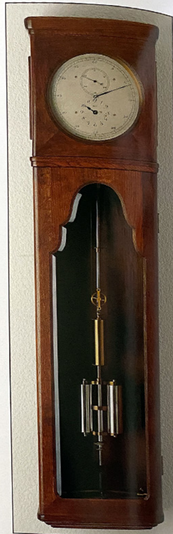
Fig. 34-20. Strasser & Rohde No. 887. This oak cased regulator, case style 11, with Type B movement, employs "Pfeiffer's Pendulum Motor" which impules the suspension every second. The nickel-steel pendulum has a brass tray for small regulating weights. There is a dead beat escapement with sapphire pallets.
