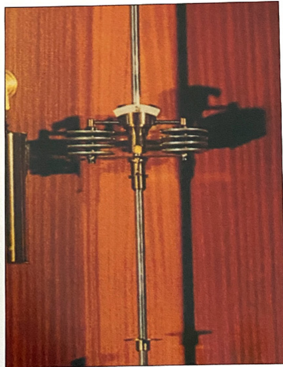
Fig. 34-13. Strasser & Rohde's aneroid compensation for barometric pressure employing two symmetrically placed units to avoid unbalancing the pendulum.
