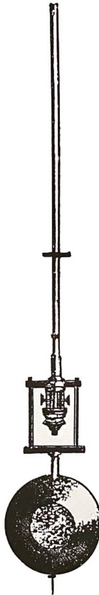
Figs. 34-8J, K (number 9). This pendulum (left) is similar to that in Fig. 8H but the compensation unit is more complex, consisting of tubes of different metals to achieve the correct level of compensation.
