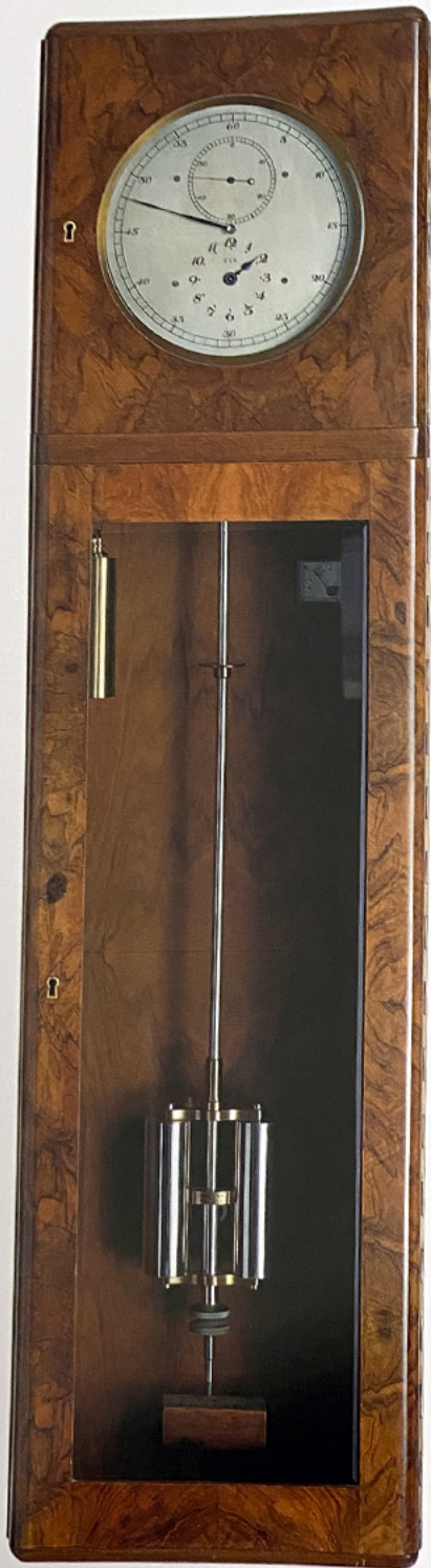
Figs. 34-23A, B. Strasser & Rohde, Glashütte, No. 713. A walnut cased wall regulator with Strasser's spring impulse escapement, offset driving weight and Invar pendulum with auxiliary compensation between the two cylinders.
