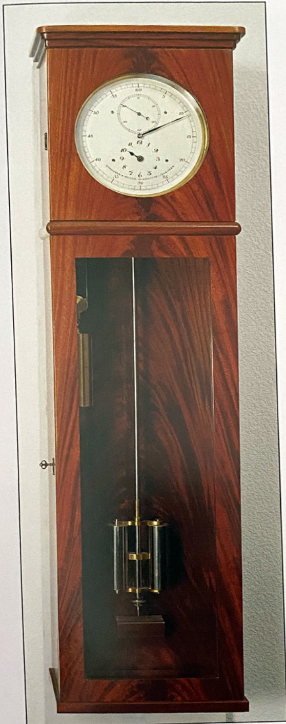
Fig. 34-17. Strasser & Rohde No. 935 in a fine mahogany No. 1 pattern case having a Type A movement with Strasser's escapement with sapphire pallets and sapphires set in chatons for the escape wheel and pallet arbors. The Invar pendulum has adjustable compensation between two cylinders.
