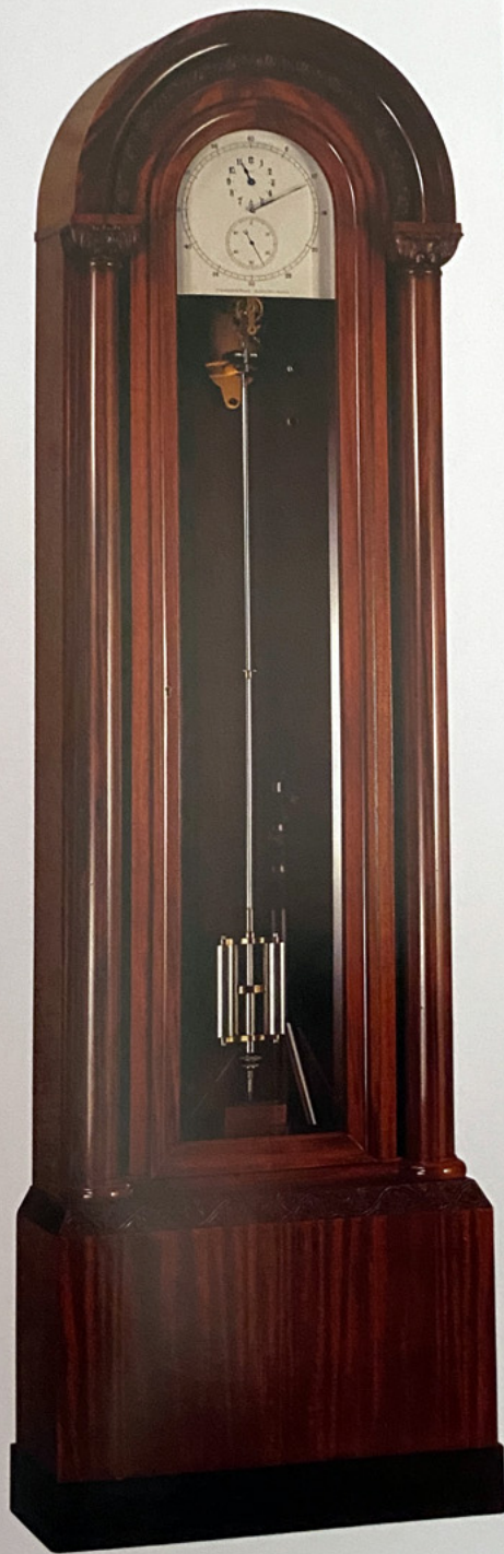
Figs. 34-24A, B. Strasser & Rohde, Glashütte, c. 1909. This regulator, in a very substantial and somewhat elaborate case, employs Strasser's inverted spring impulse escapement with jeweled pallets and his twin cylinder Invar pendulum. The close up of the escapement illustrates his form of pendulum suspension, designed to protect it from any disturbance. Musée International d'Horlogerie, La Chaux-de-Fonds.
