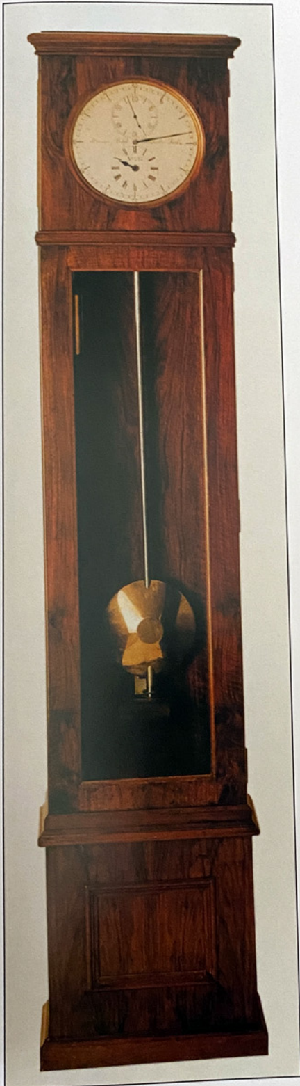
Fig. 34-26. Strasser & Rohde No. 245. This is a Type A regulator with Strasser's escapement in a modified pattern 17 walnut case, and a Riefler Invar pendulum. The four pillar movement, with jeweled pivot holes set in chatons for the escape wheel and pallet arbors, have ruby pallets. The weight is offset to the side and a four spring suspension is used.
