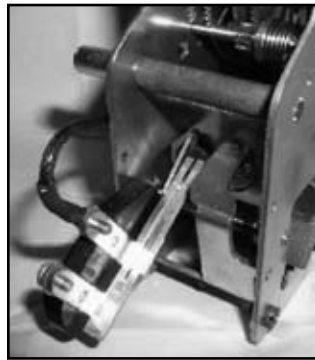
Figure 4A, left. Stromberg Model 31. Figure 4B, above. Closeup of Model 31 motor contacts.
